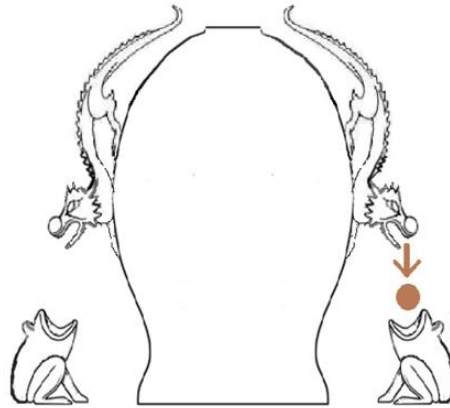
Figure 1. Zhang Heng's seismoscope, an ancient Chinese instrument for detecting earthquake direction.
