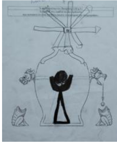
Figure 2. Student reconstruction of Zhang Heng's seismoscope based on an inverted pendulum mechanism, illustrating the release of a ball into the dragon's mouth according to Newton's First Law of Motion.
